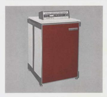
The  $\mu$ -COMP DDP-416 general purpose digital computer offers a price/performance ratio that can't be beat: full size 16-bit capability, nano-second speeds, I/C size/reliability, ASCII compatibility, wide instruction repertoire and simple memory addressing.
