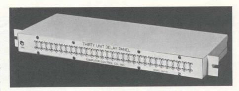
in series by simple taper pin jumper connections to form the desired total delay. The basic one-microsecond delay interval per line, accurate to within ±2 percent, can be used directly with the other Series T modules. Where large amounts of electrical delay are required in a minimum physical volume, the Model DU-10 affords an ideal solution. It is also useful for many other compu-
